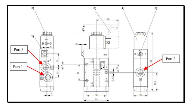
The solenoid valve is Normally Open (NO) when port 2 is connected to port 3. For normal operation of the pump, the air-supply will be connected to port 2 and taken from port 3. When the solenoid valve receives and electrical signal (activated), the air supply will go to port 1. Port 1 should be connected to a vent away from personnel.
